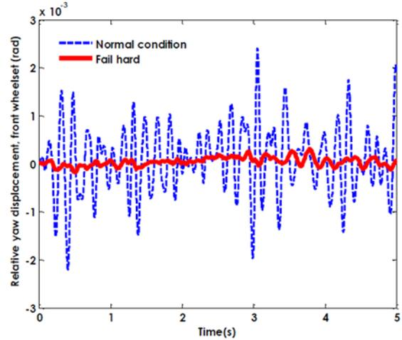
Figure 4: Displacement due to yaw for the forward-facing wheel (FH)
