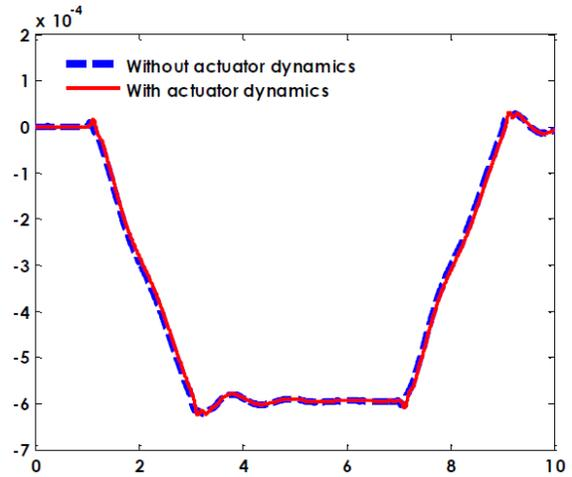
Figure 2: Angle of attack with and without actuator dynamics
