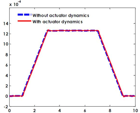
Figure 1: lateral displacement with and without actuator dynamics
