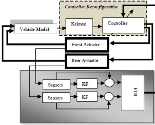
Figure 3: Schematic diagram of the FDI system
