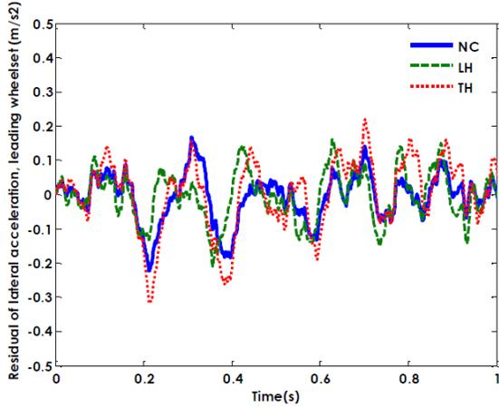
Figure 6: lateral acceleration residual values of the front wheel
