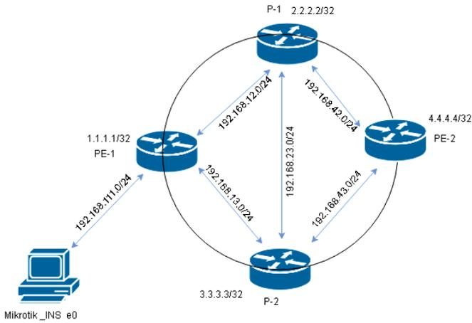
Figure 3: showing the test topology used for the testing of Mikrotik virtual OS and its performance
