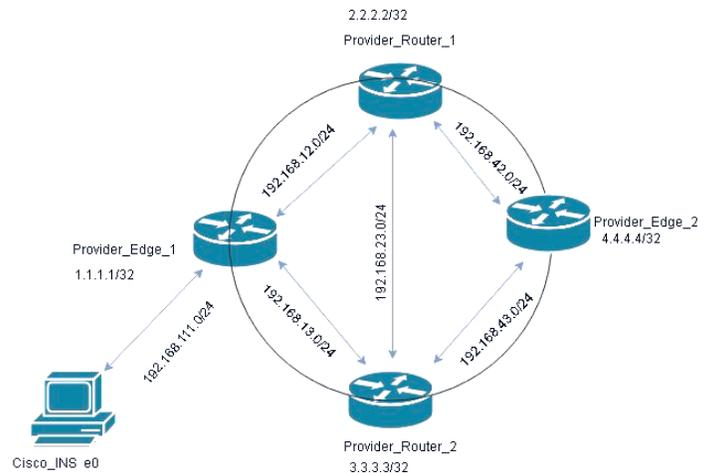
Figure 2: showing the test topology used for the testing of Cisco and its performance graph
