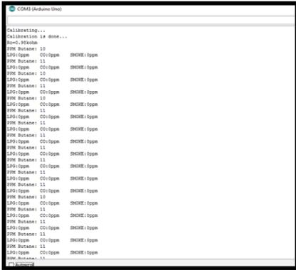
Figure 8. PPM values in Serial Monitor at Normal State
