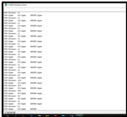
Figure 9. PPM Value Higher than Threshold in Serial Monitor
