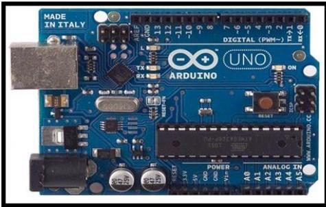
Figure 4. Arduino hardware
