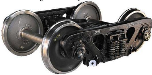
Figure 3. Wheelset arrangement in a bogie: Courtesy to [5]
