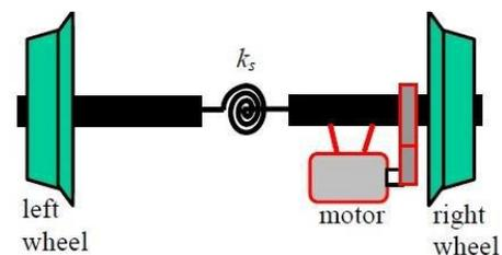
Figure 1. Motor mounted wheel set: Courtesy to [9]
