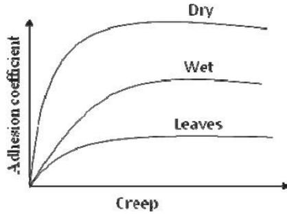
Figure 2. Adhesion Curves: Courtesy to [3]
