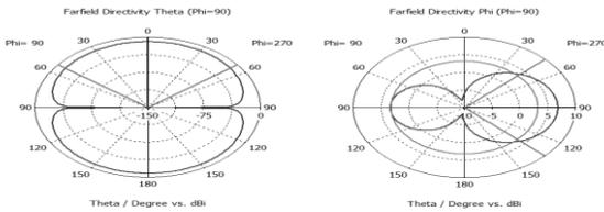
**Max radiation at  $E_\theta = 0^\circ$  &  $E_\phi = 90^\circ$  ( $S1=ON, S2=ON$ )**
