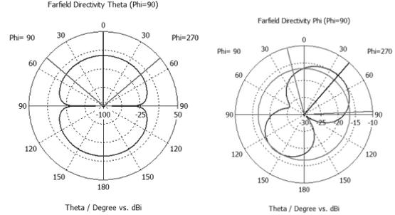
Max radiation at  $E_0 = 0^\circ$  &  $E_\phi = 41^\circ$  (S1=OFF, S2=ON)
