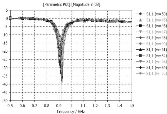
Fig-5 Variation in the S11 parameter with change in the area of substrate
