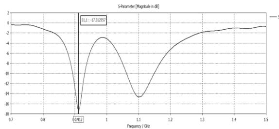
Fig-10 Return Loss when Both Switches are in ON states
