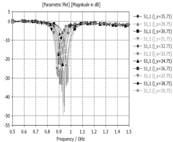
Fig-7 Variation in the S11 parameter with change in the length of the dipole
