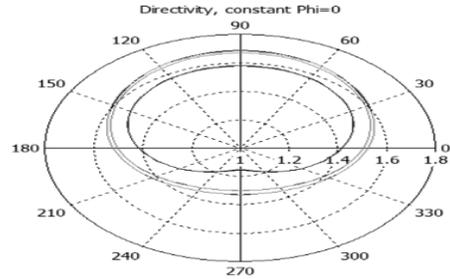
**Fig-13 Optimized maximum directivity of reconfigurable antenna at  $\phi=0^\circ$**
