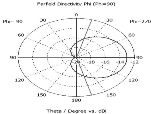
Fig-4 Antenna directivity in H-Plane (maximum at  $E_{\theta} = 90^{\circ}$ )
