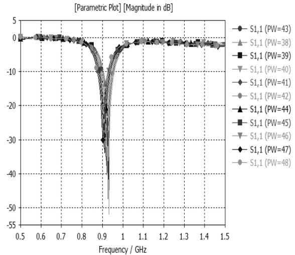
Fig-6 Variation in the S11 parameter with change in the area of patches
