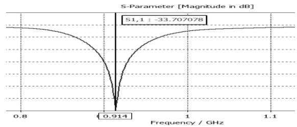
**Fig-2 Return Loss or S11 Parameter of single band antenna**
