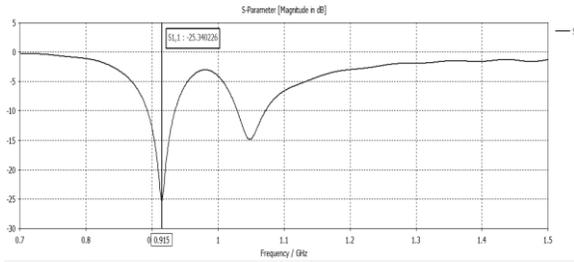
Fig-9 Return Loss when one of switch is ON
