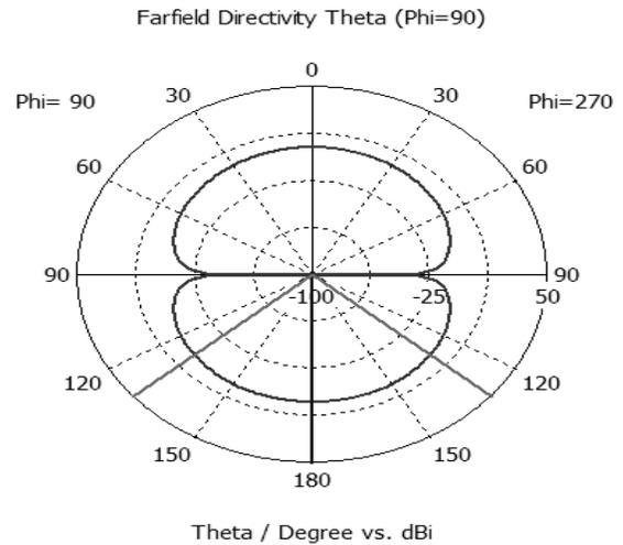
**Fig-3 Antenna directivity in E-Plane (maximum at E<sub>θ</sub> = 180°)**
