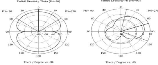
**Max radiation  $E_\theta = 0^\circ$  &  $E_\phi = 69^\circ$  ( $S1=OFF, S2=ON$ )**
