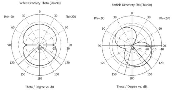
Max radiation at  $E_0 = 180^\circ$  &  $E_\phi = 139^\circ$  (S1=ON, S2=OFF)
