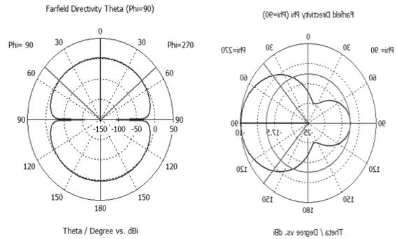
Max radiation at  $E_0 = 0^\circ$  &  $E_\phi = 90^\circ$  (S1=ON, S2=ON)
