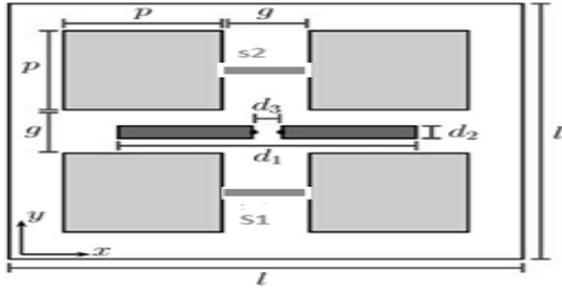
Fig-8 Geometry of Reconfigurable Patch Antenna
