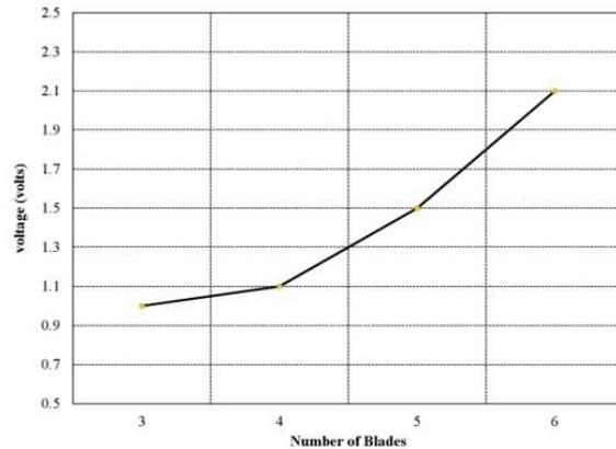
**Fig. 2. Number of Blades vs Output voltage characteristics**
