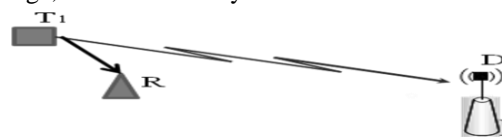
Fig. 3(a). Relay : 1st phase of the transmission
