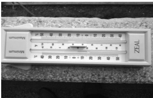
A small type of Thermometer used in the Field
