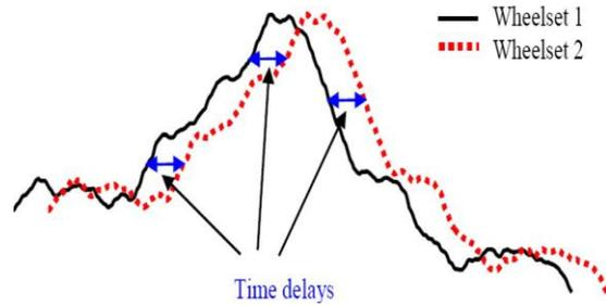
Figure 2 Movement of wheels due to track roughness.
