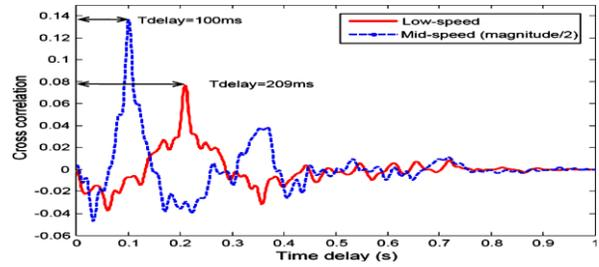
Figure 7 Resulting Cross correlation of the productive motions at 46, and 95.32 km/h
