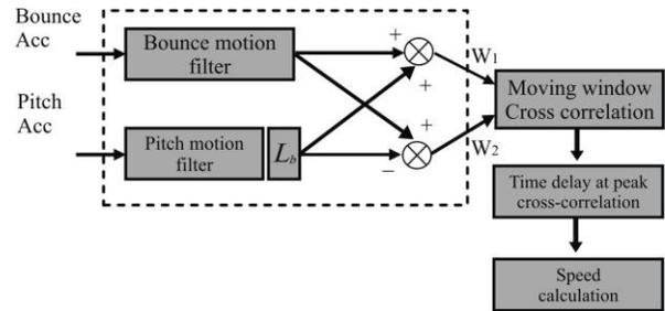
Figure 3 Speed measurement scheme.
