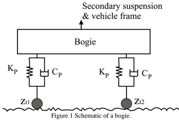
Figure 1 Schematic of a bogie.
