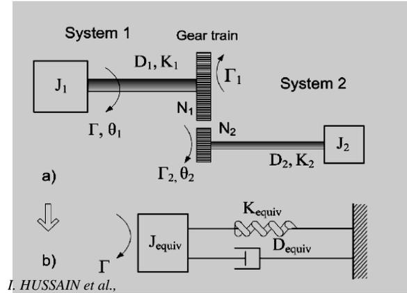
**Fig. 1: Drive Train Model of wind Turbine**
