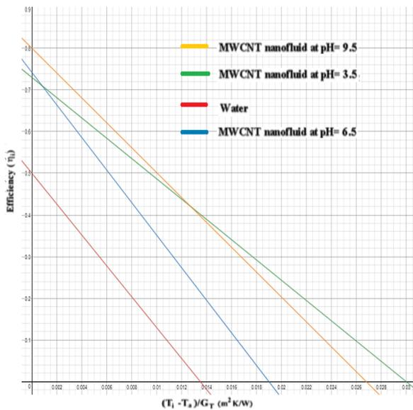
Fig. 05. MWCNT nanofluid as base fluid at three pH values as compared with water in 0.0333 kg/s mass flow rate
