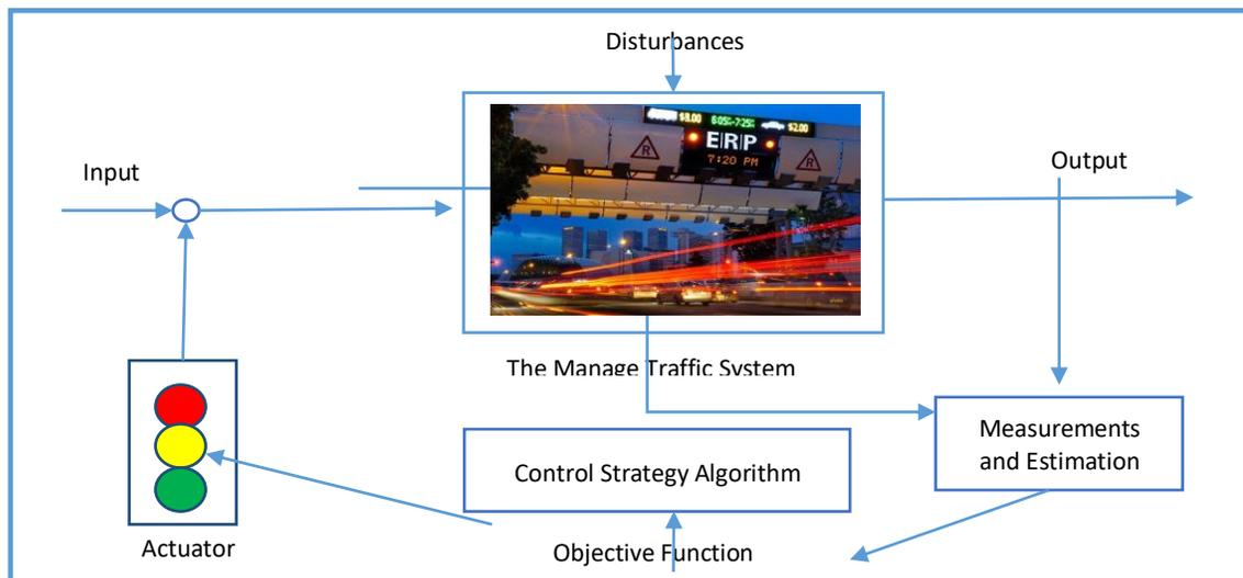
Fig. 2: Block diagram of the controlled traffic process (Prachi, Kasturi, and Priyanka 2014)
