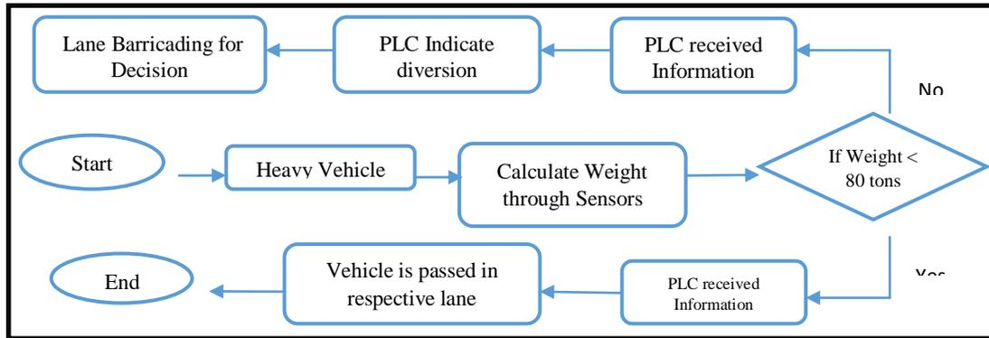
Fig. 1: Flow chart for diversion of vehicles based on weight
