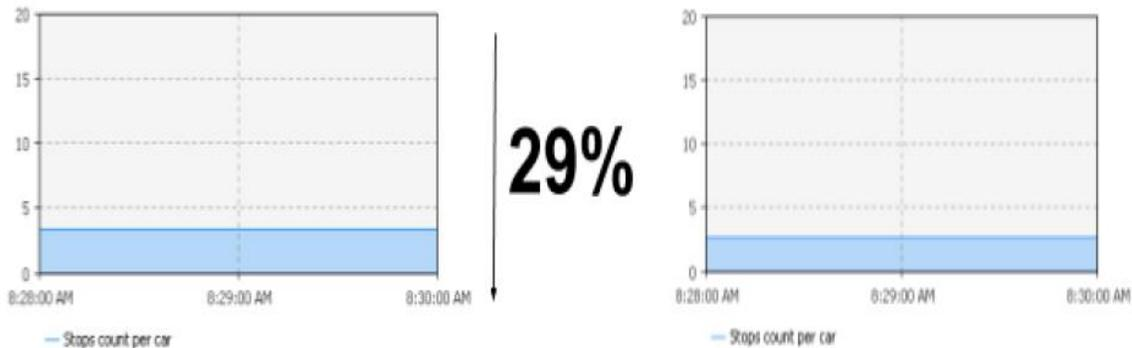
Fig. 10: Stops count per car in traditional system vs smart system
