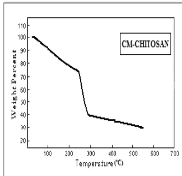
Fig 1. Thermogravimetric Analysis of Carboxymethyl Chitosan
