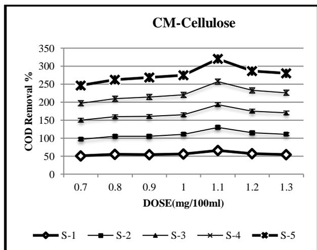
Fig 4: The optimum dosage (mg/100) for COD removal % of municipal waste water
