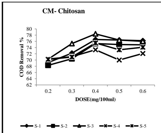
Fig 3 : The optimum dosage (mg/100ml) of CM-Chitosan on COD removal % of municipal waste water sample
