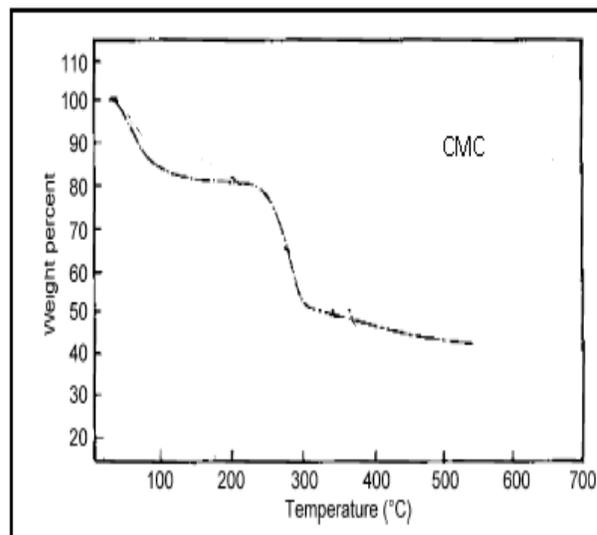
Fig. Thermogravimetric Analysis of Carboxymethyl Celluloses
