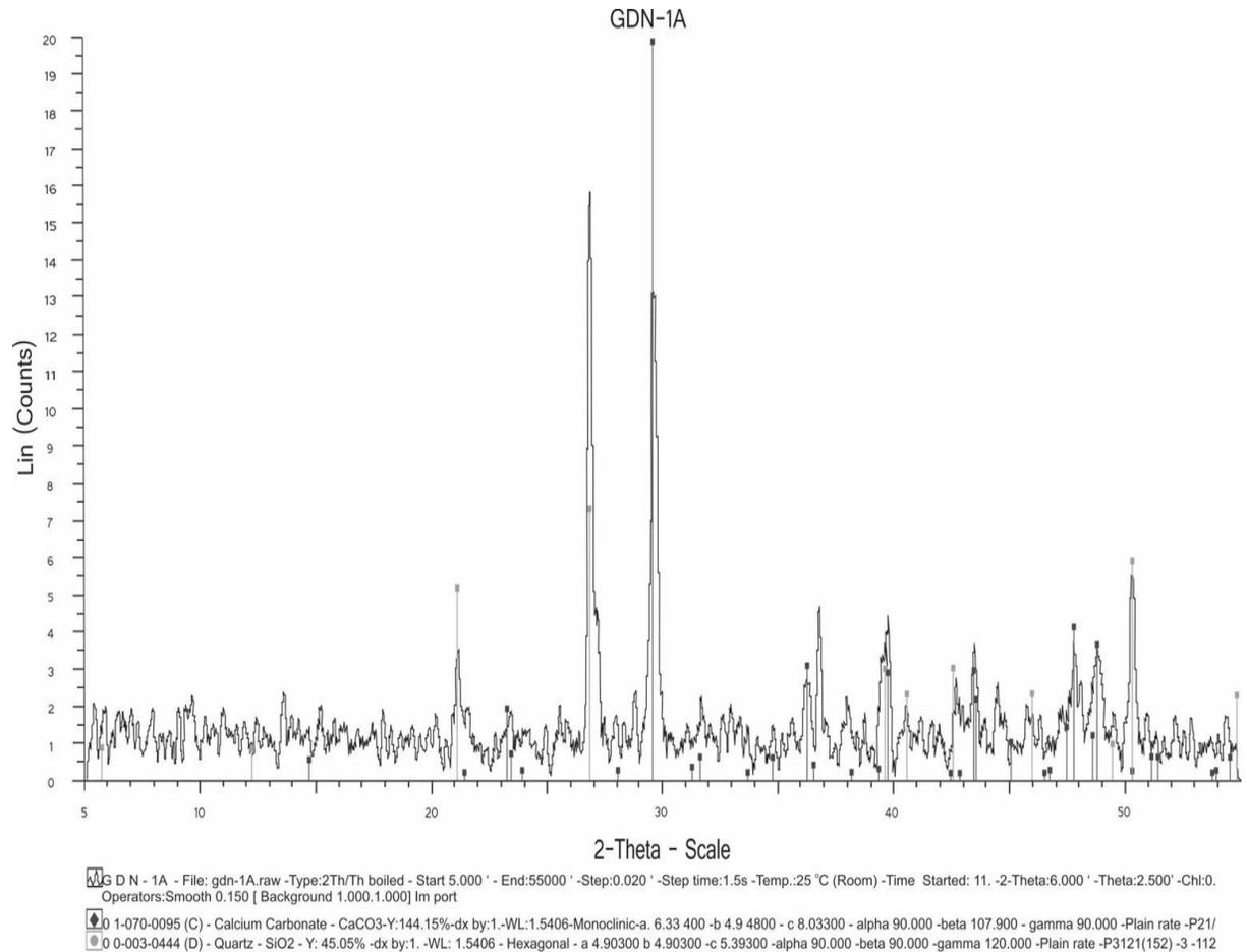
Fig. 4. XRD diffractogram of sample GDN-1A showing the concentration of different minerals specially; Quartz and Calcite.
