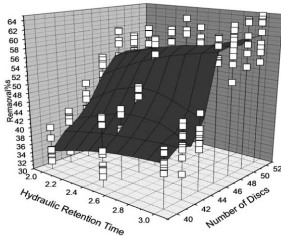
Fig. 1. Response Surface effect of Retention Time and Number of Discs on Removal of Chemical Oxygen Demand
