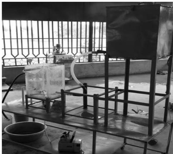
Fig. 1: DAF Apparatus
