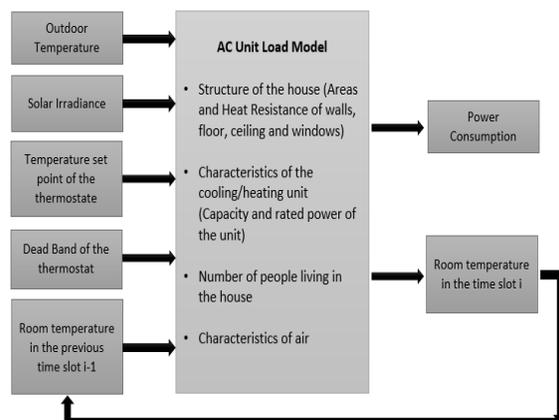
Fig. 2: AC Load Model
