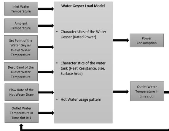
Fig. 1: Water Geyser Load Model
