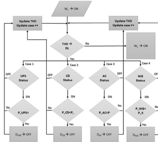
Fig. 5: EMS algorithm's flow chart in accordance with loads priorities level
