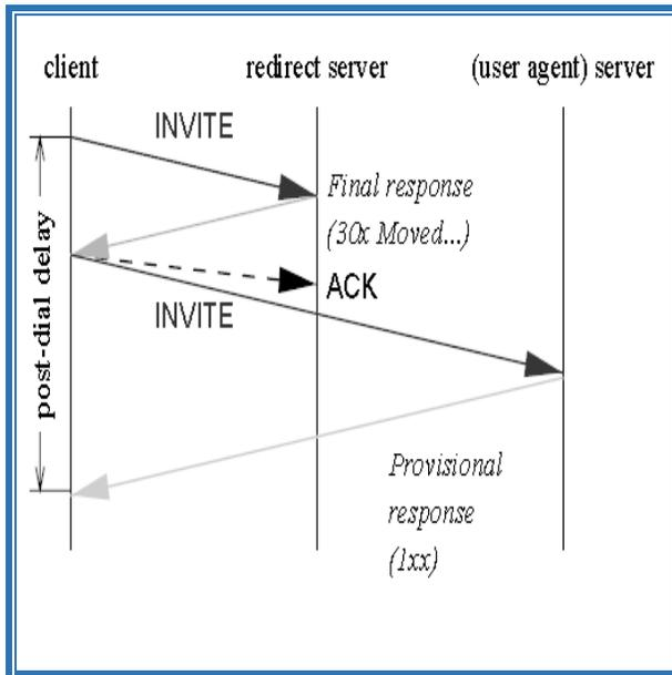
**Fig.6. Ack: return for call initiation (RTP)**
