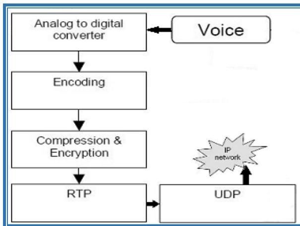
Fig. 5. Basic Voice flow in VOIP system
