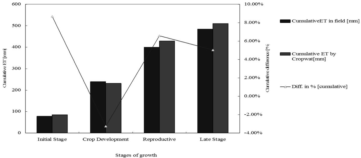
Fig.2 Comparison of cumulative ET measured in field and calculated by Cropwat.
