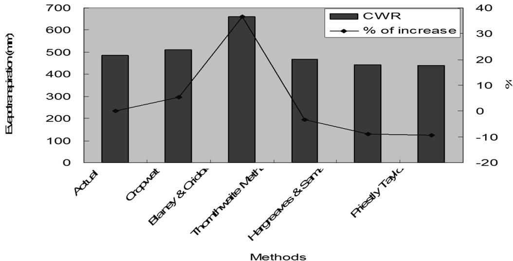
Fig. 3. Measurement and Prediction of Crop Water Requirements
