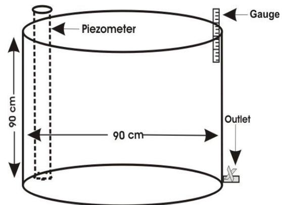
Fig. 1 Schematic layout of the container
