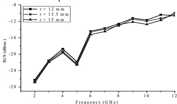
Fig.6. Effect of r on RCS of the modified antenna
