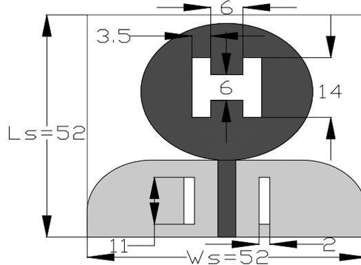
Fig.2 (a).The Geometry of modified antenna
