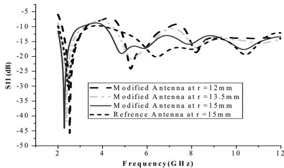
Fig.3. Comparisons of return loss curves of the reference antenna and modified antenna at different size of patches
