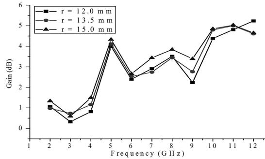
Fig. 4. Effect of r on gain curves of the modified antenna
