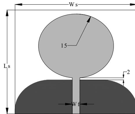
Fig.1 (a).The geometry of reference antenna
