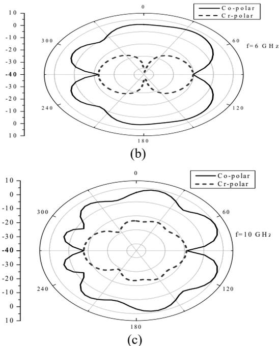
Fig. 5. The simulated co-polar and cross polar radiation pattern of the modified antennas at  $\theta=90^\circ$  in xy-plane for frequencies of (a) 2 GHz (b) 6 GHz (c) 10 GHz
