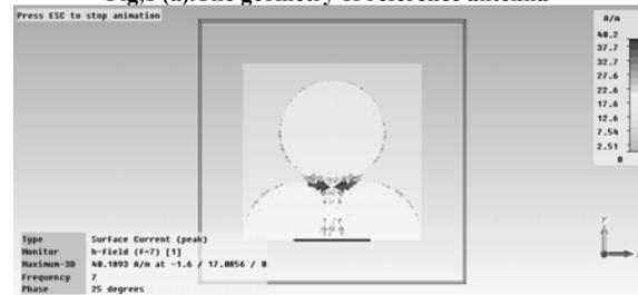
Fig.1 (b) The Surface current distribution of referenced antenna
