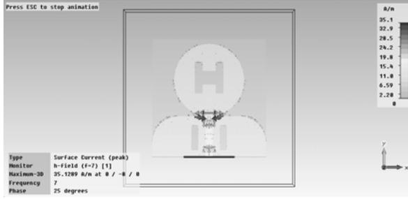
Fig.2 (b).The Surface current distribution of modified antenna
