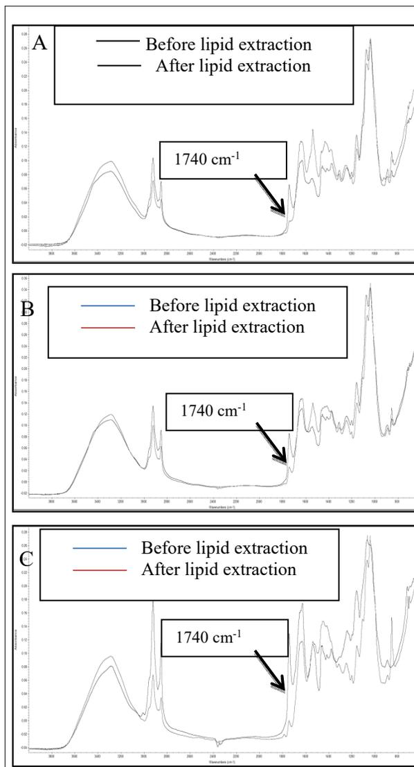
**Fig. 1:** FTIR spectra of *Nannochloropsis oculata* measured on (A) Day 9, (B) Day 12 and (C) Day 14
