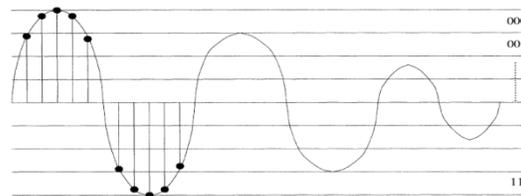
**Fig 6: Sampled Waveform**
