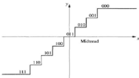
**Fig 7: Quantized Waveform**
