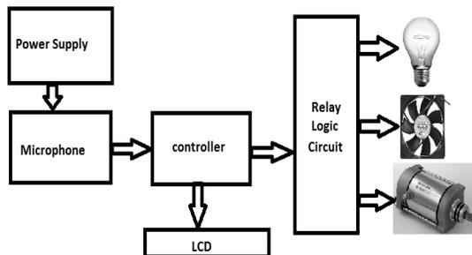
**Figure2: Block diagram of controlling devices through voice recognition**
