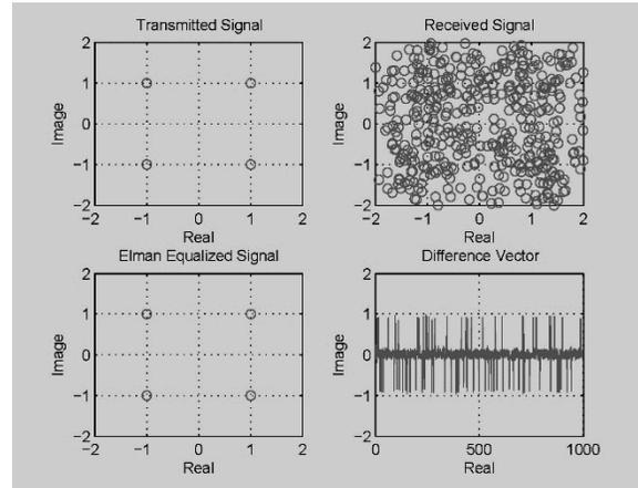
**Fig. 8 Summarized transmitted, received and Elman equalized output**
