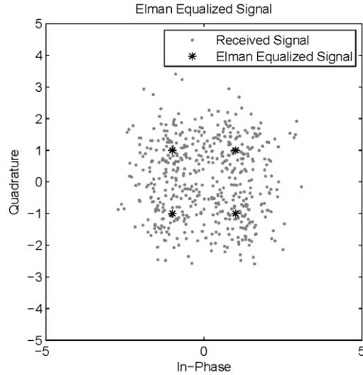
**Fig. 7 Scatter plot of received signal and Elman equalized output**
