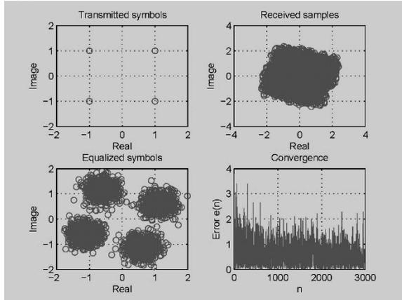
Fig. 11 Performance of CMA algorithm as an equalizer
