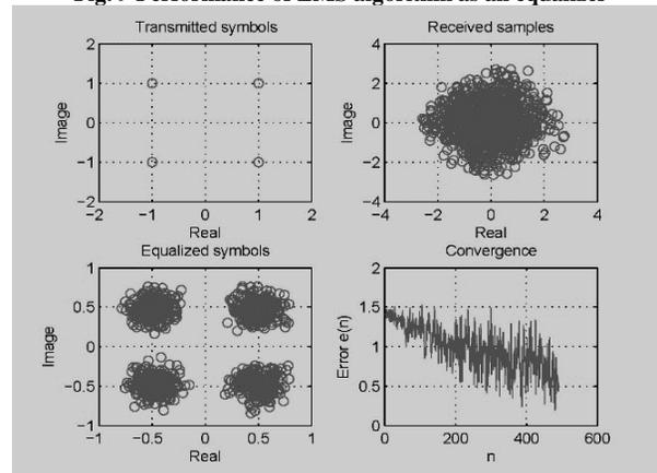
Fig. 10 Performance of ZF-MMSE Algorithm as an Equalizer
