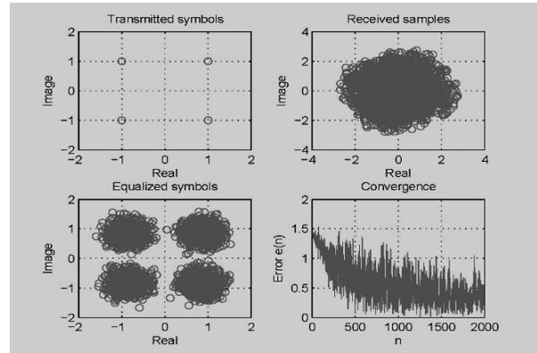
Fig. 9 Performance of LMS algorithm as an equalizer
