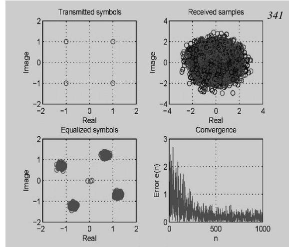
Fig. 12 Performance of adaptive CMA in fractional space based equalizer
