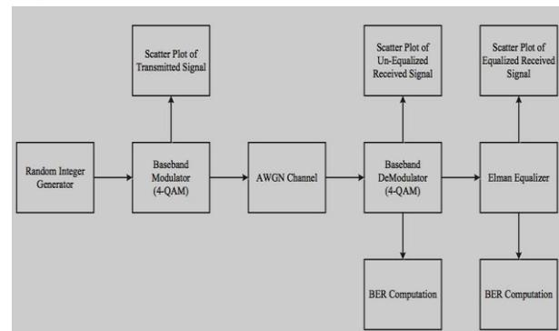
Fig. 3 Block diagram of channel equalization using Elman Network
