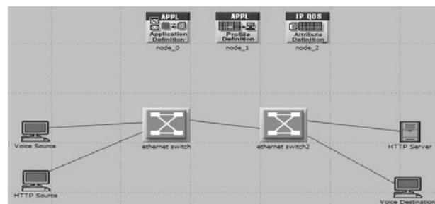
Fig 1: Using IP topology for VoIP
