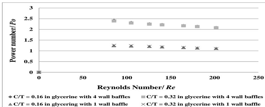
Fig. 6: RCI power numbers with 1 or 4 wall baffles and at two clearances in glycerin.
