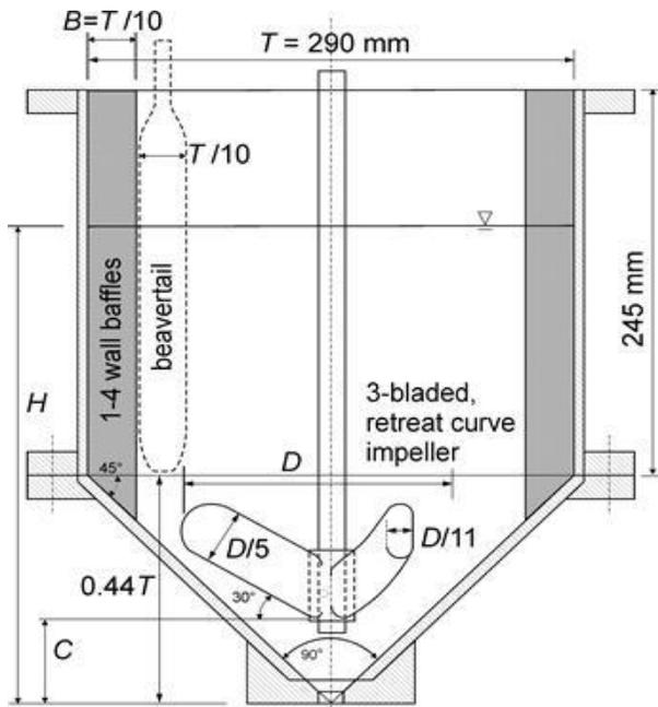
Fig.1: The geometry of the conical based STR, retreat curve impeller, wall baffles and a beavertail baffle.
