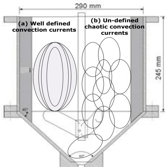
Fig. 2: Well defined and chaotic flow visualised inside the RCI powered STR.
