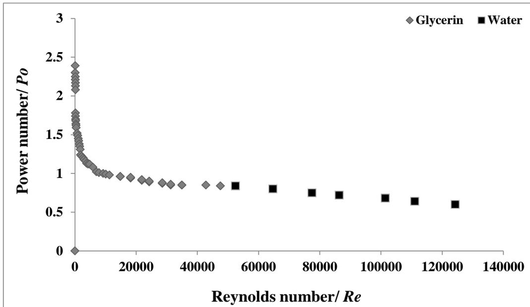
Fig. 3: Power number vs Reynolds number for varying viscosity glycerine and water in the conical based STR with four wall baffles and  $C/T=0.32$ .
