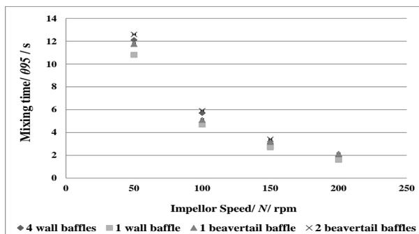
Fig. 8: Effect of baffle arrangements on the 95% mixing time at various speeds for the RCI in a conical-based vessel.
