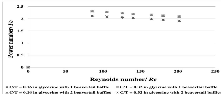
Fig. 7: RCI power numbers with one and two beavertail baffles and at two clearances.
