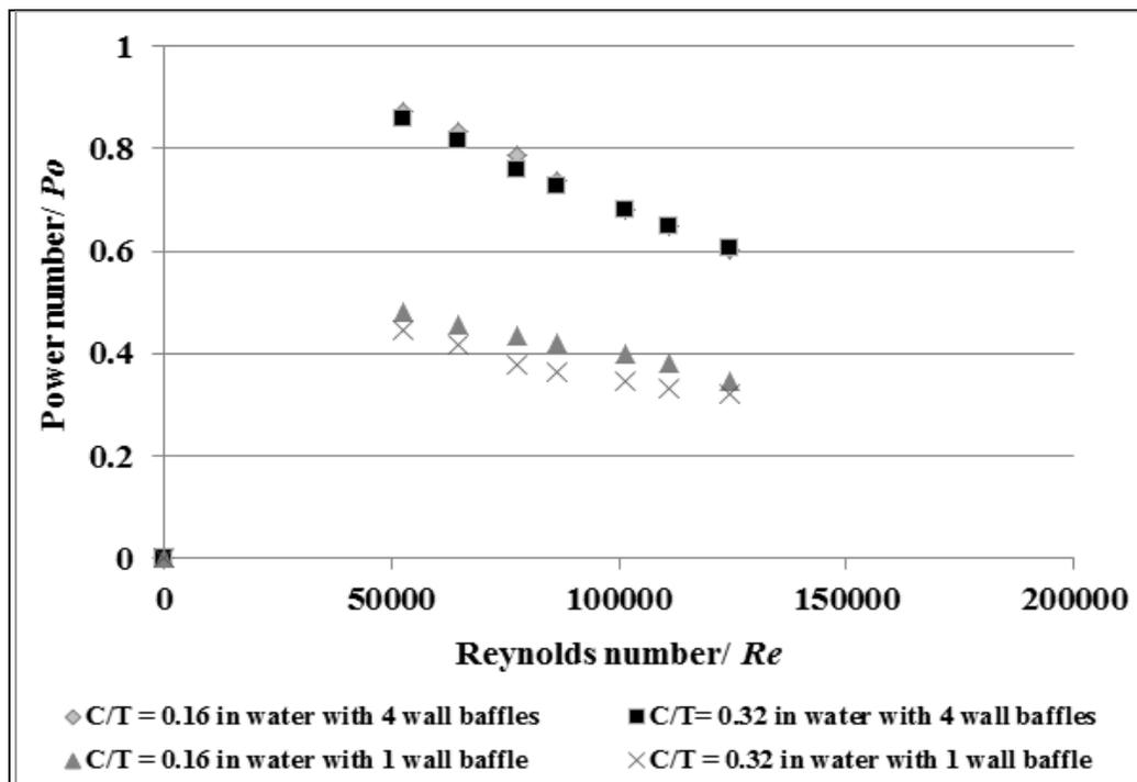
Fig. 4: RCI power numbers with 1 or 4 wall baffles and at two clearance with water.
