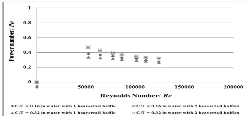
Fig. 5: RCI power numbers with a single and two beavertail baffles at two clearances in water.
