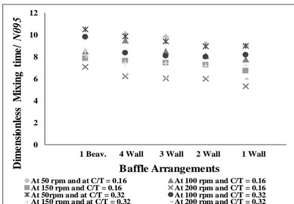
Fig. 9: Dimensionless mixing times for various baffle arrangements at two impeller clearances with water as working fluid.
