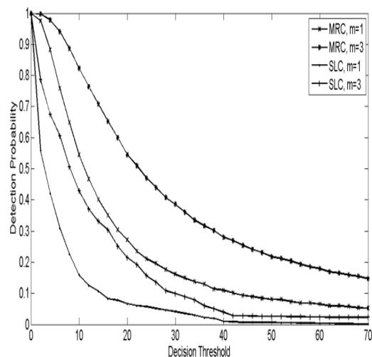
Fig. 4: Detection Probability for MRC and SLC Schemes with  $n=3$  over Nakagami fading channels ( $m=1$  and  $m=3$ )
