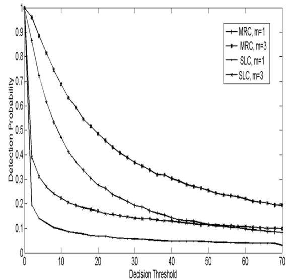
Fig. 3: Detection probability for MRC and SLC Schemes with  $n=1$  and direct path over Nakagami fading channels ( $m=1$  and  $m=3$ )
