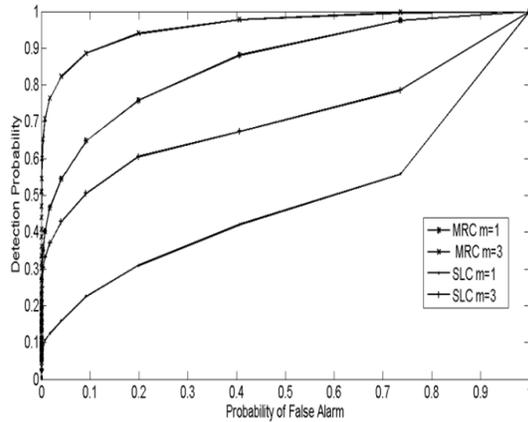
**Fig. 5: Detection probability variations with probability of false alarm for  $n=3$  relays using MRC and SLC Schemes.**
