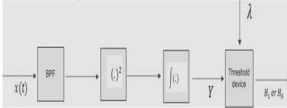
Fig. 2: Block diagram of Energy Detector
