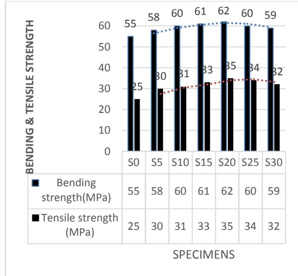
Fig 5 Variation of tensile and bending strength with change in NMF weight ratio
