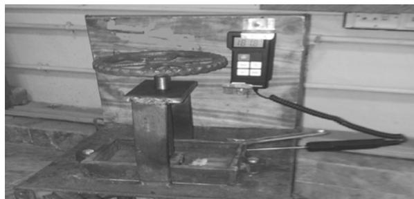
**Fig. 1. Flat plat pressing mould for PCB-PVC composites processing**
