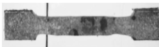
**Fig. 2. Standard shape for tensile test**
