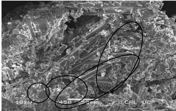
**Fig. 7** SEM photograph of 500 micron NMF of PCBs
