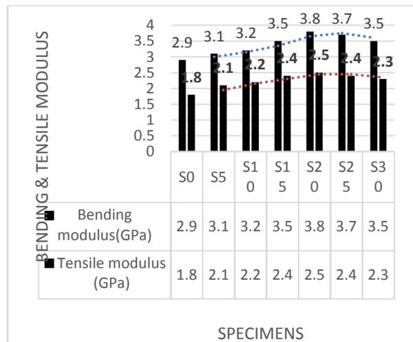
Fig 6 Variation of tensile and bending modulus with change in NMF weight ratio
