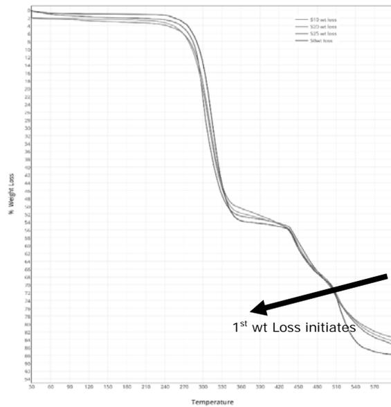
Fig. 4 Combined TGA cures of PCB-PVC composites
